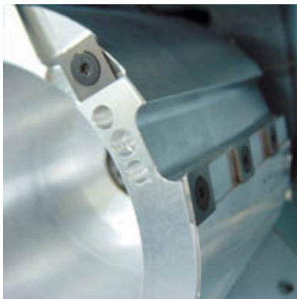
New cutter head with reversible carbide tips for extreme machining rates and optimum chip removal.
