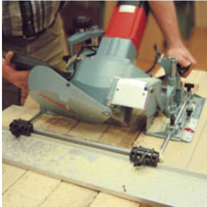
The ZK 115 Ec with the guide rail.
