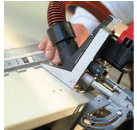
Quick and economical: Making carcasses with the DD40 and dowel template.
